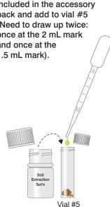
4. Cap vial and shake occasionally for 30 seconds during the 30 minutes extraction period.
